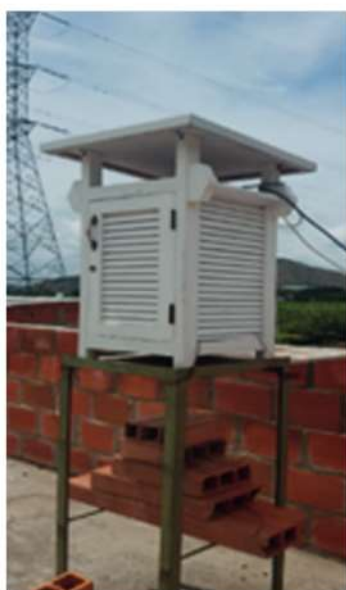
Fig. 2. Thermometric box used to protect the PM 2.5 sensors.
