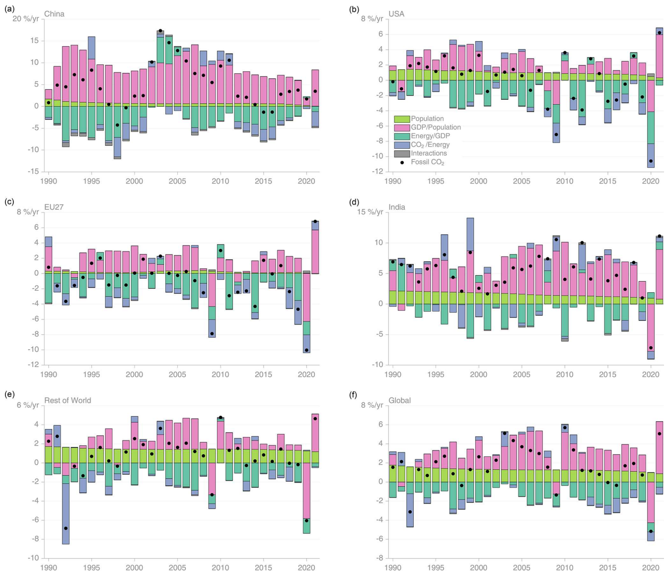
Figure 15. Kaya decomposition of the main drivers of fossil CO 2 emissions, considering population, GDP per person, energy per GDP, and CO 2 emissions per energy, for China (a), the USA (b), the EU27 (c), India (d), the rest of the world (e), and the world (f). Black dots are the annual fossil CO 2 emissions growth rate, coloured bars are the contributions from the different drivers. A general trend is that population and GDP growth put upward pressure on emissions, while energy per GDP and more recently CO 2 emissions per energy put downward pressure on emissions. Both the COVID-19-induced changes during 2020 and the recovery in 2021 led to a stark contrast to previous years, with different drivers in each region.
