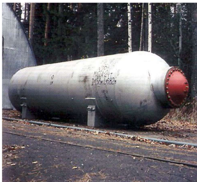
Fig. 8 A KOLBA chamber outside its storage bunker at the former Semipalatinsk Test Site. The diameter is 2.4 m and the length is 7 m. It was made of steel reinforced with Kevlar and fiberglass. Source: Siegfried Hecker. Page 27 in “Plutonium Mountain” published by Belfer Center at Harvard Kennedy School. (2013)
