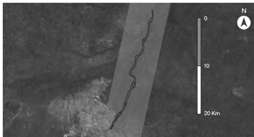
Figure 7. Virtual station (in red) leading to unreliable water level time series. The orientation of the river bed follows the S3 satellite track (in purple) over almost 30 km. For each date, all pulse observations falling into this geometry are averaged introducing artifacts due to great variations occurring along the river.
